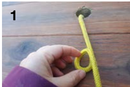
1 Tie the top end of a rope securely to your load (the hole) Make a loop in the rope.
